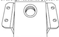
Position against the upper wall (resistance of approx. 30.9 lbs / 14 kg)
